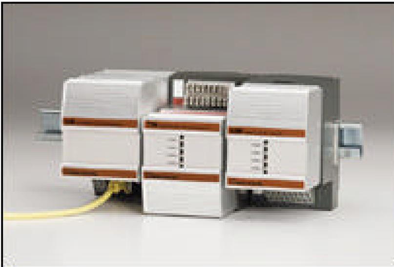
The NCS system uses a Ethernet Interface Module (EIM) (the left-hand module with the ethernet CAT5 cable connected) to allow communication between the two input/output modules to its right and the operator and/or programmer through the human machine interface (HMI). That HMI can be either a third party-supplied package, a custom-written Visual Basic / Visual C++ application, and many others.
