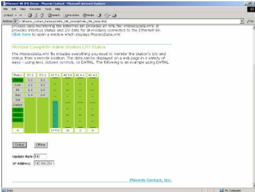
This is a dynamic html webpage that shows the status of all of the Phoenix Contact FactoryLine I/O. In each of the seven columns, the colors will change depending upon the status of the I/O. For example, as the analog input PV changes, the bar graph in column 4 will raise or lower. In columns 2 and 3, as the digital inputs and outputs change the grey squares will change to green if the I/O points are energized. The left-most column shows the status of the interface module.
